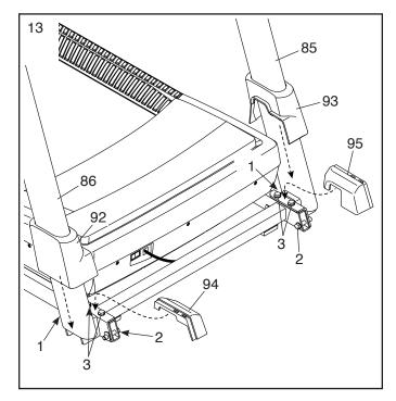
14. Make sure that all parts are properly tightened before you use the treadmill. If there are sheets of plastic on the treadmill decals, remove the plastic. To protect the floor or carpet, place a mat under the treadmill. To avoid damage to the console, keep the treadmill out of direct sunlight. Keep the included hex keys in a secure place; one of the hex keys is used to adjust the walking belt (see page 29). Note: Extra hardware may be included.
