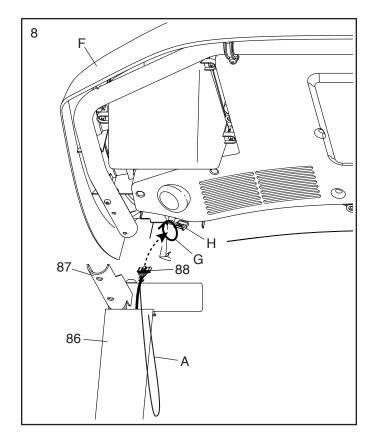
9. Set the console assembly (F) on the Right and Left Handrails (81, 80); do not pinch any wires.
